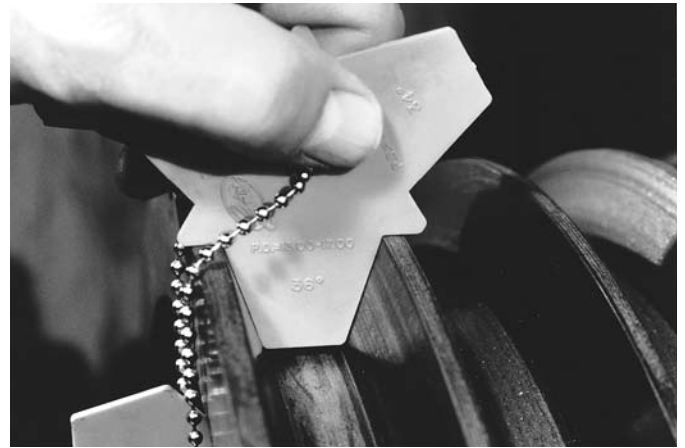
Pulley gauges make wear detection easier.
